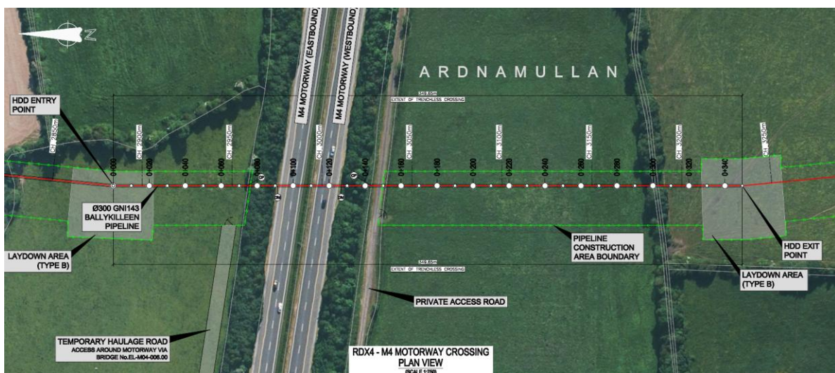
Figure 36: Plan View of the proposed HDD Crossing and Pipe String Corridor at the M4 Motorway Crossing (refer to drg. no. GNI143-GNI-PL-CRD-0003-01).
