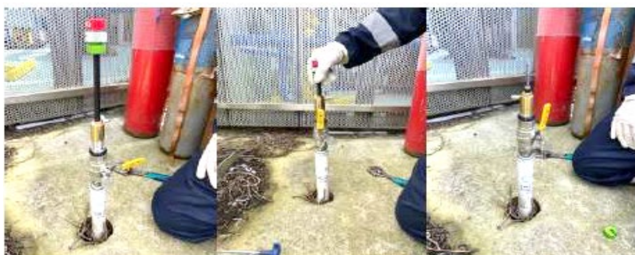
Figure 2-2: Field Trial Demonstration of Mechanical Stopper at GNI Training Centre, Dublin.
